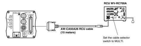
() Before proceeding to connect the RCU to the camera, set the RCU's power switch to OFF.
